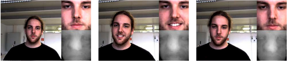
Fig. 5. Result of the data preparation phase: Three different depth images of the same person aligned to a frontal position (aligned color/depth image in resp. right column)
