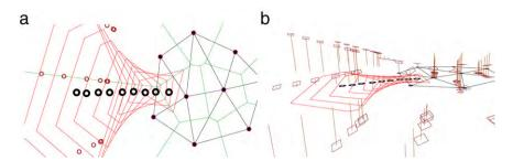
**Fig. 7.** (a) The virtual tile evolution for evaluation positions (drawn as thick rings) moving away from the data sites, with ghost points (small rings) moving away as well. (b) Perspective 2.5D view of the setting from (a), the gradients shown as tilted rectangles placed at the data sites.
