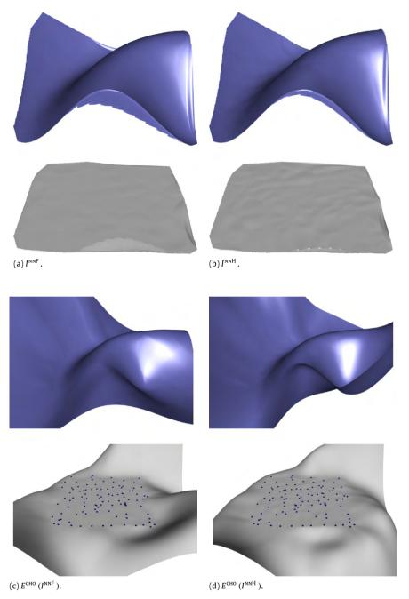
**Fig. 15.** (a), (b) Farin's and Hiyoshi's interpolants applied to the data set. The artifacts in the front and on the right side are clearly visible. (c), (d) Both interpolants augmented by the CHO ghost point strategy. An interesting result is the apparently worse performance of the  $C^2$  interpolant in terms of wriggles.
