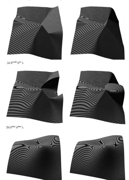
Fig. 10. (a), (b) The discontinuous change of the interpolant in *D* is propagated to  $D^{E}$ . (c) Wendland's RBF interpolant is independent of any triangulation.
