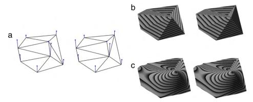
**Fig. 9.** (a) Two almost identical data sets, with different tessellations. (b) Linear interpolation in the underlying triangulation, the discontinuous change of the interpolant due to the edge flip is clearly visible. (c) Farin's C<sup>1</sup> interpolant does not have this problem.
