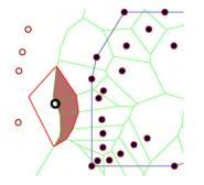
**Fig. 4.** Illustration of sub-tiles used in the dismissed ghost point method. The areas of the shaded polygons are used to determine the affine weights by which to mix the values at the corresponding data sites (drawn solid).
