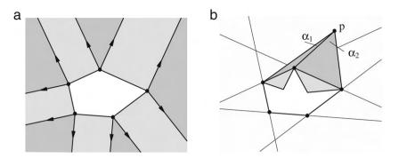
**Fig. 2.** (a) Partition of the complement of the convex hull into cones and half-open prisms (wedges and half-open rectangles in 2D), as used in  $E^{\text{AKI}}$  and  $E^{\text{FRA}}$ . (b) To evaluate at **p** using  $E^{\text{ALFB}}$ , the functions from the light gray triangles adjacent to the convex hull are extrapolated and mixed based on the angles  $\alpha_1$  and  $\alpha_2$ .
