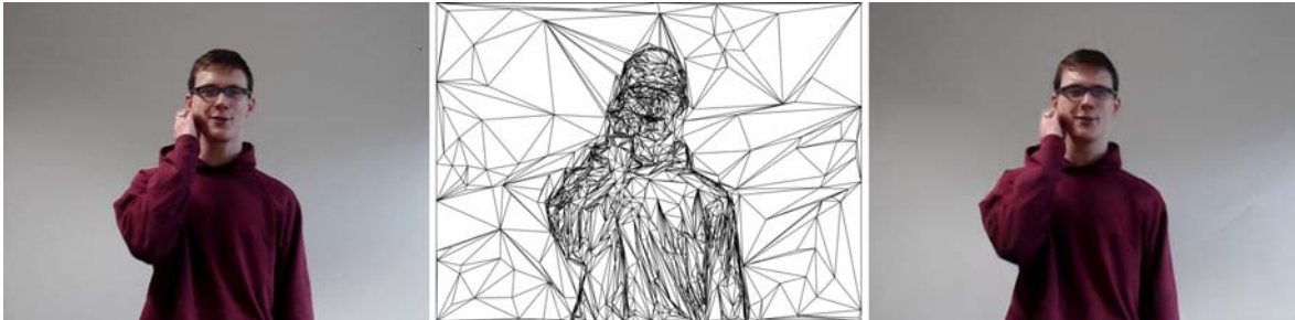
Figure 1: Video \mathbf{V} compressed with 1500 vertices per frame: original frame f_i (left), triangulation t_i (middle), approximation A_{t_i} (right).
