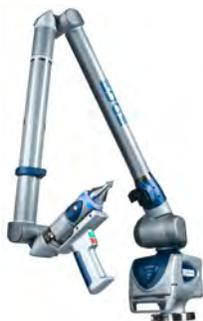
Fig. 1: FARO Edge ScanArm (www.faro.com, 09/25/2015)
