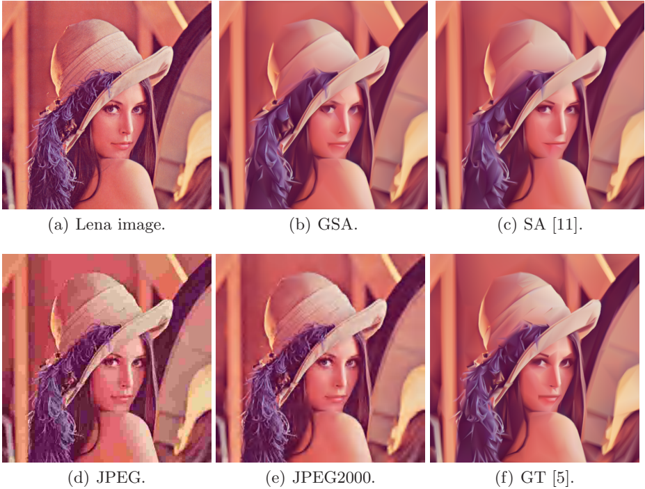
Fig. 7. Original image ( \sim 770 kB) (a), and approximations ( \sim 5750 bytes) using GSA (b), SA [11] (c), JPEG (d), JPEG2000 (e), and GT [5] (f), (courtesy USC SIPI)
