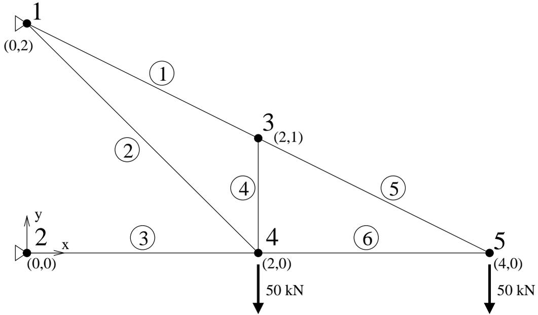
Figure 1: Mechanical Truss Model with Six Elements
