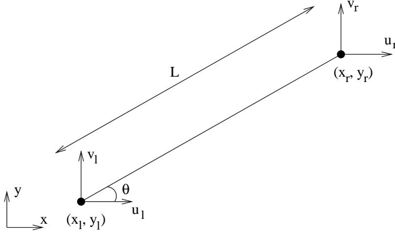
Figure 2: Arrangement of a Single Element Connecting Left-Hand and Right-Hand Nodes
