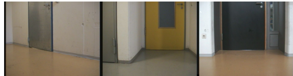
Figure 1: Illustrates typical door images, taken by the robots camera. The top of the doors are occluded and also the diversity of doors are recognizable: The doors have different poses, colors, lighting situations as well as different features e.g. door gap or texture on the bottom.
