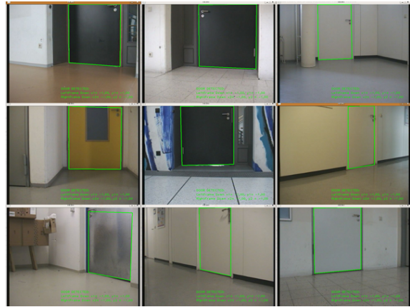
Figure 6: Typically by the AdaBoost classifier detected doors. The pictures demonstrate that our approach is robust against different robot positions, reflection situation as well as different door features.
