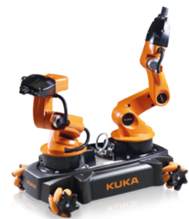
KUKA youBot omni-directional mobile platform with two 5-degree-of-freedom manipulators with two 2-finger grippers
