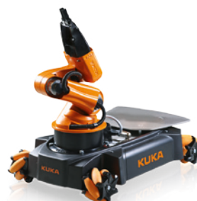
KUKA youBot omni-directional mobile platform with 5-degree-of-freedom manipulator with 2-finger gripper
