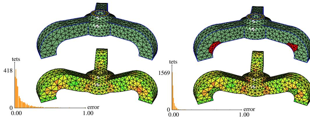
■ **Figure 6** Adaptive subdivision and FE simulation. First column: tetrahedral base mesh (2,799 tetrahedra) and simulation with visualization of the approximation error (green=low – red=high) and the histogram of the error distribution; second column: adaptively refined mesh (4,540 tetrahedra) showing the refined regions in red, and simulation results for the once adaptively refined mesh.
