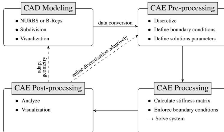
■ **Figure 1** Different phases in the modeling and simulation process.
