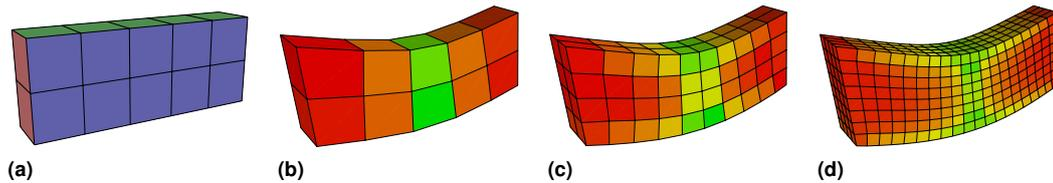
■ **Figure 8** (a) Base mesh of model to be simulated. Red faces are fixed, to green faces a load is applied. (b) Simulation of base mesh, (c) simulation of once refined mesh, (d) simulation of twice refined mesh. For the visualization of the stress the same scale is used as in Figure 6.
